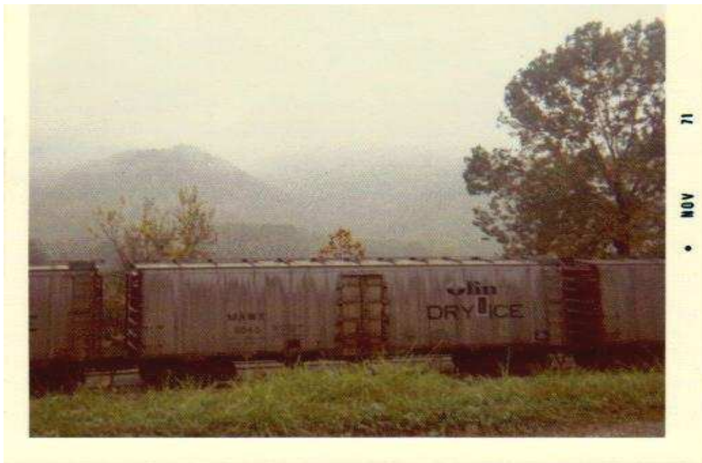
Olin Mathieson Reefer used for shipping dry ice from the Saltville, VA, plant. According to a former worker at the Norfolk & Western yard at Saltville where this picture was taken in November 1971, Olin shipped several of these 40 footers each day with dry ice. Photo by Mike Jackson.
