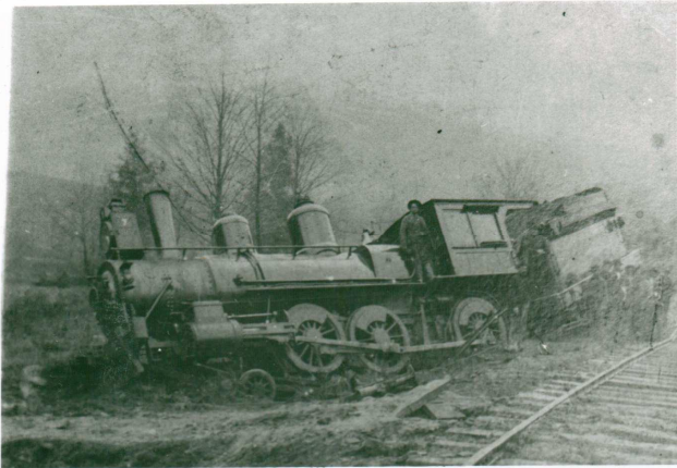
Upper left: M&RV No.7 jumped a the track at a high rate of speed, just outside the town of Marion. An improperly lined switch was to blame.
