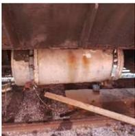
**“Clinchfield 100” office car (WATX 100):** New water system and tank (left photo) along with a new 142-gallon fuel tank being added to the car.
